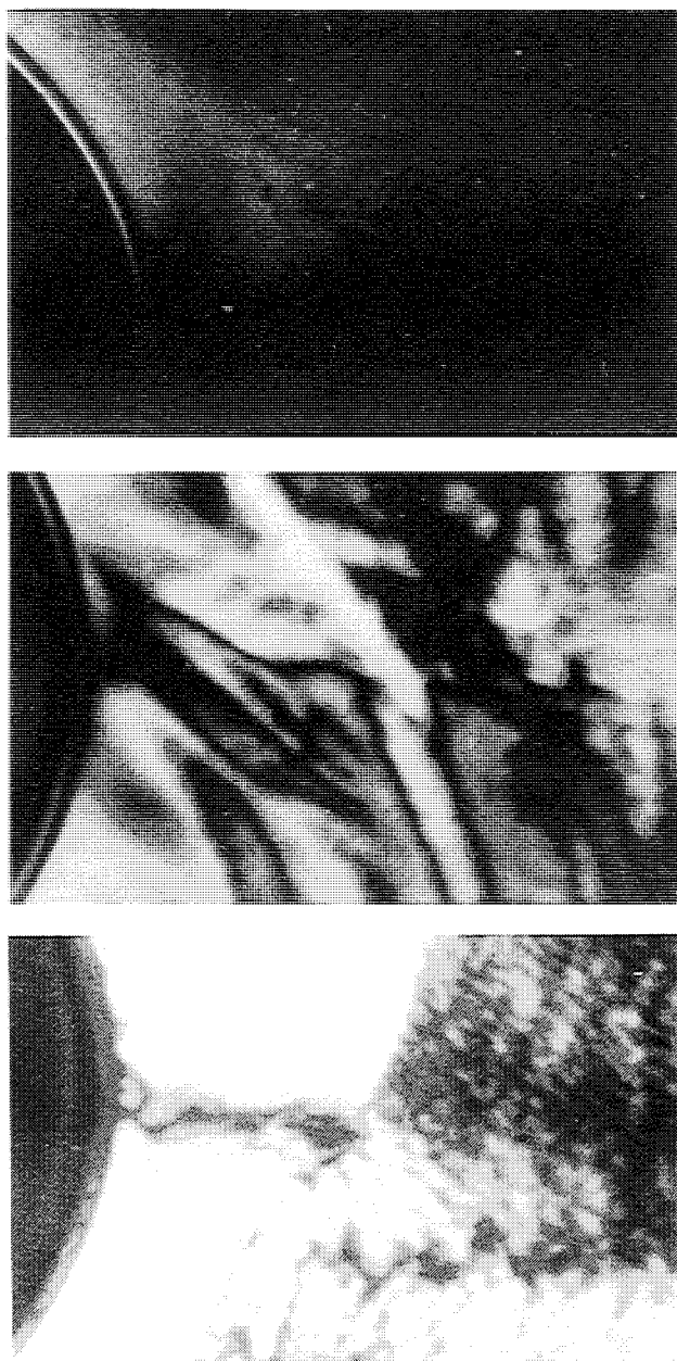
Figure 2. Effect of NaCl on liquid crystal formation of 4 mg/mL deterelix after 3 weeks at room temperature. These micrographs were made under crossed polarized light. The left part of the slide is air only (no formulation buffer) and thus is dark. The curved meniscus separates the air phase from the formulation phase containing birefringent liquid crystals (shown as intense white). Various NaCl concentrations were used: top, 1.5 mM; middle, 7.5 mM; bottom, 15.4 mM.
